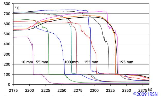
Temperature during reflooding of a 4mm debris bed with 200W/kg power deposit inside
