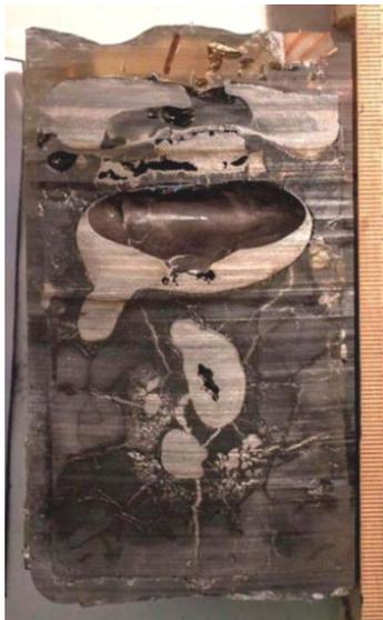
*Evidence of steel transfer across the oxide crust and thinning of top metal layer (from NITI)*
